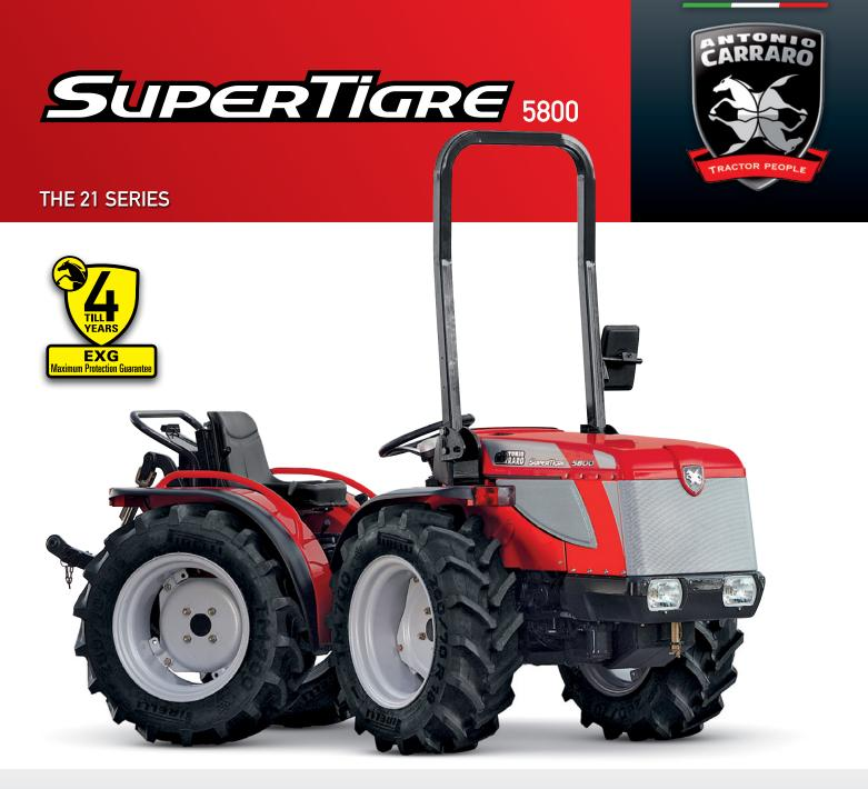
The **Supertigre 5800** is a new equal wheel tractor from the unbeatable Series 21. Designed for work on hillsides and mountains and specialised crops. Four equal wheel drive, optimum weight-power ratio, reduced steering angle all mean stability and constant traction on all types of terrain along with a capacity for quick manoeuvrability and disengagement.
