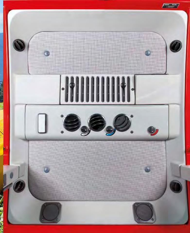
The incoming air is cleaned by a large filter, with an available activated carbon filter\*.
