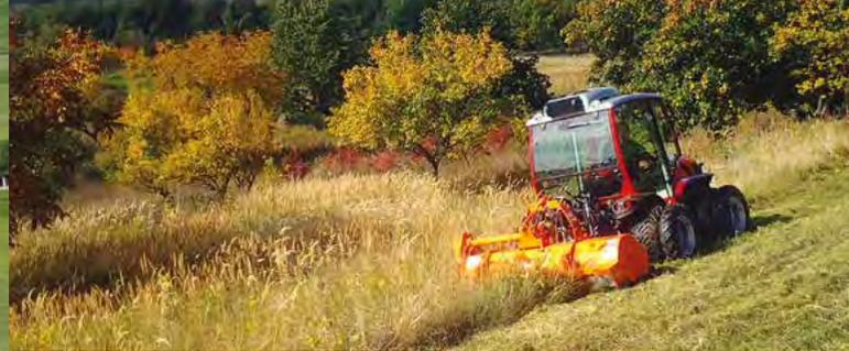
Mower, excavator, loader, fork-lift, baler, sower, planter, tiller, reach mower, snow blower and blade, grass cutter, trailer, sprayer and shredder, are just some of the more common implements that can be used with the Ergit 100 series TTR tractors. The tires are interchangeable, as every type of terrain requires its own tire that can optimize tractor performance.
