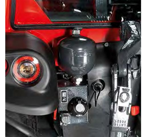
Hydropneumatic suspension with automatic pressure control.
